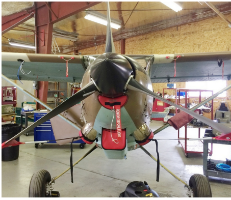
Siai Marchetti 1019 Engine Plugs, Prop Tie-Exhaust Covers
