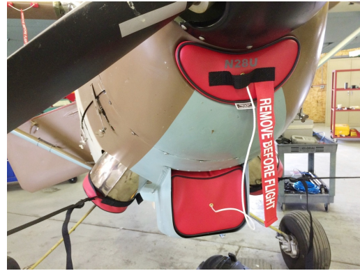
Siai Marchetti 1019 Engine Plugs, Prop Tie-Exhaust Covers
