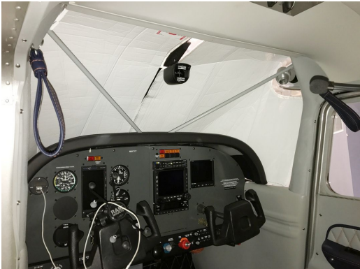
Cessna 180 Skywagon Windshield Heatshield, (W/ Compass)
