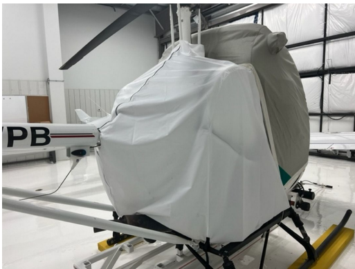
Schweizer 300C Engine Cover, test fit cover
