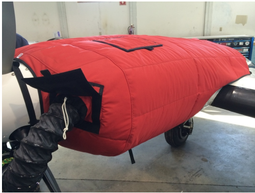
Cessna 402 Insulated Engine Cover with Heater
