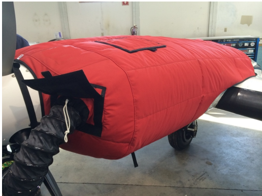
Cessna 402 Insulated Engine Cover with Heater
