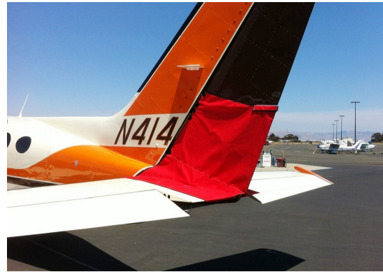
Cessna 414 Rudder Openings Cover (bird barrier)
