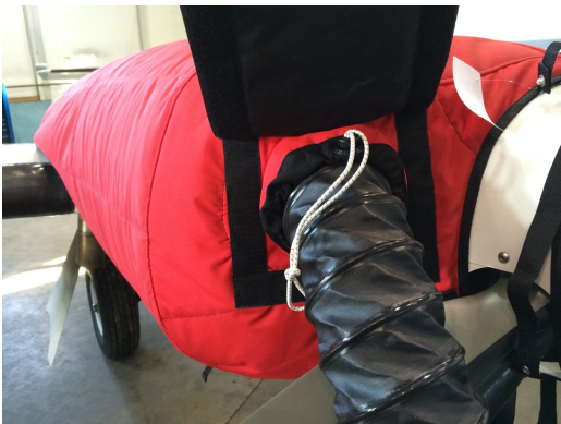
Cessna 402 Insulated Engine Cover with Heater
