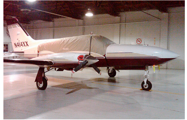
Cessna 414 Canopy Cover and Engine Inlet Plugs
