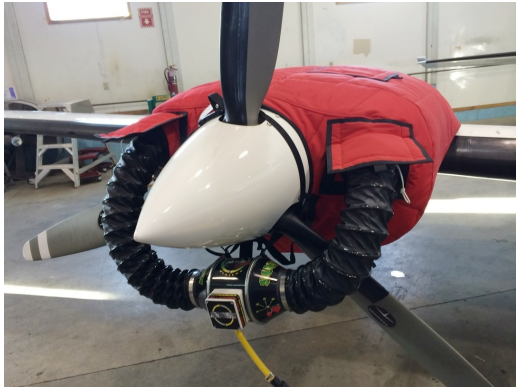
Cessna 402 Insulated Engine Cover with Heater
