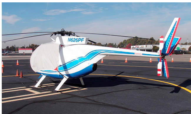
MD500C Bubble Cover with Wire Strike detail
