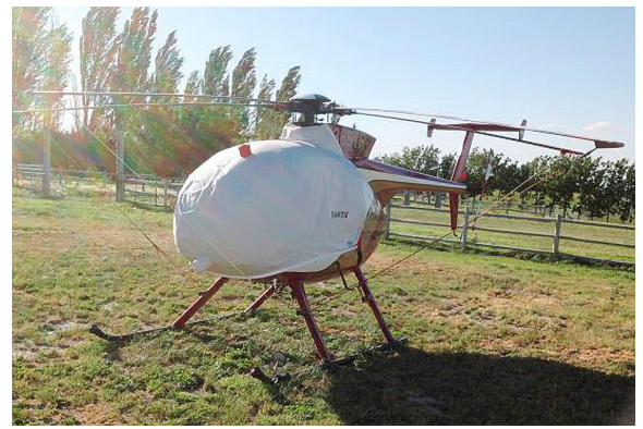
MD500D Bubble Cover with Intake Add-On
