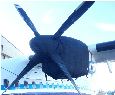
ATR-72-202 Insulated Engine & Prop Hub Covers
