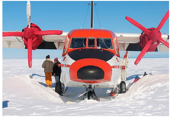
Casa 212 Insulated Engine & Propellor/Spinner Covers
