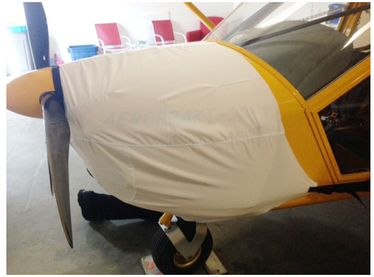
A-22 Engine Cover, test fit
