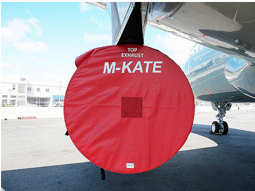
Airbus A319 Intake/Exhaust Covers set, IAE V2500
