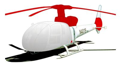
Gazelle Bubble, Abbr. Engine, Rotor Hub, Blades & Fenstron Covers (Illustration)
