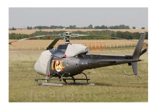
Airbus Helicopter AS350 Bubble Cover & Intake/Exhaust Cover
