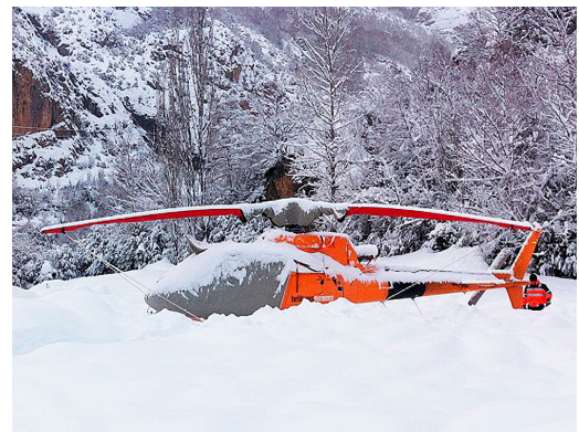
AS350 Bubble Cover, Insulated Main & Tail Rotor Covers, Blade Covers with tie-down detail
