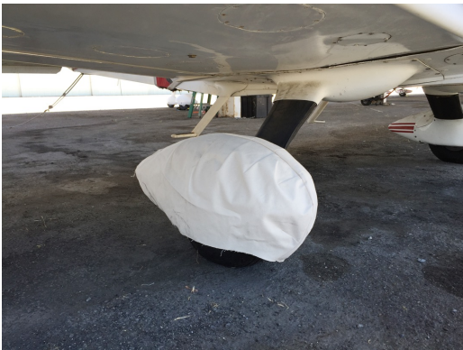
Grumman AA5 Main Wheelpant Cover, test fit
