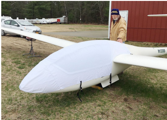
Grob 102 Astir CS Canopy/Nose Cover (test fit)
