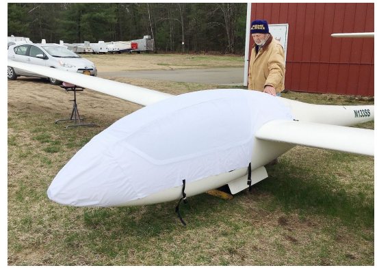
Grob 102 Astir CS Canopy/Nose Cover (test fit)
