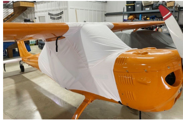
Aeromarine Merlin Over-Top Canopy Cover, test fit cover
