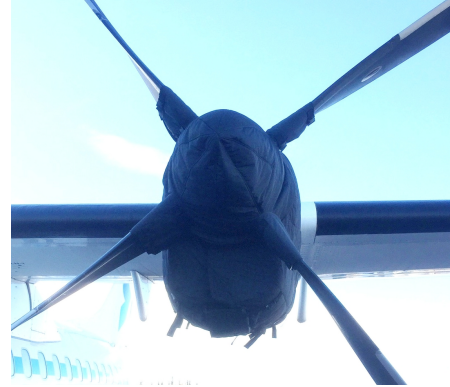
ATR-72-202 Insulated Engine & Prop Hub Covers
