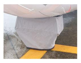
ATR-42/72 Nose Gear Landing Gear/Tire Covers
