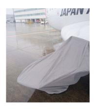
ATR-42/72 Main Gear Landing Gear/Tire Covers
