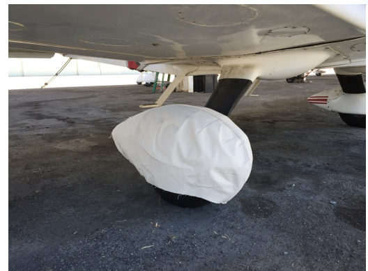
Grumman AA5 Main Wheelpant Cover, test fit
