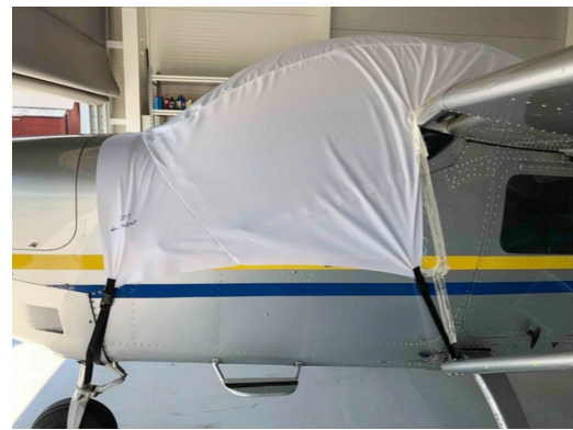
Saab Safari Canopy Cover, test fit cover
