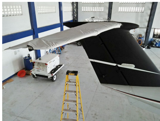
Beech King Air B350 Horizontal Stabilizer Covers
