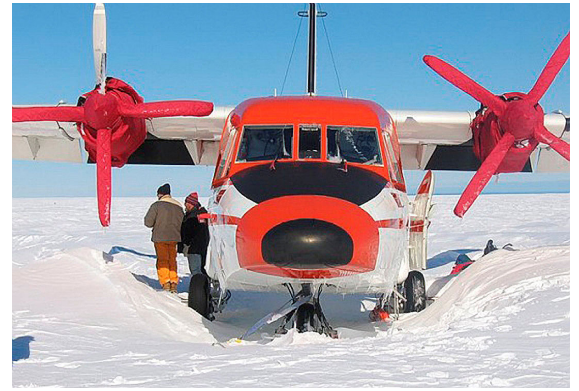
Casa 212 Insulated Engine & Propellor/Spinner Covers
