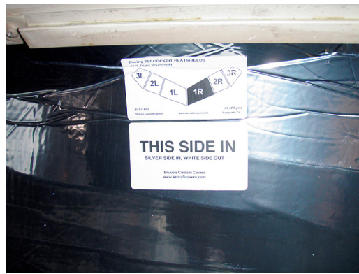
Boeing 757 Cockpit HeatShield set, installation detail
