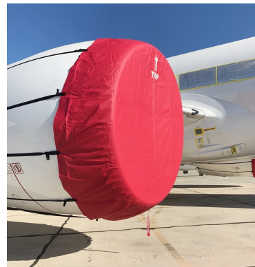
Boeing 787 Dreamliner Intake Covers Kit, Oem Type, Each, Boeing P/N: K10011-1 (Equals Qty 2 Of K10011-2), Adjustable Straps To Bypass Attachment Detail
