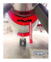
Engine and Oil Cooler Inlet Plugs
