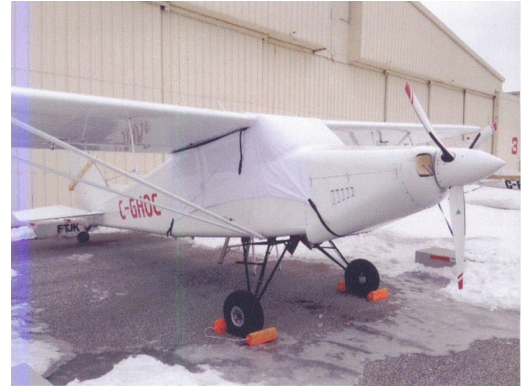
Bushcaddy Canopy Cover, test fit cover
