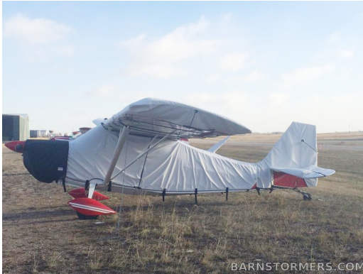
Bellanca Citabria Extended Canopy Cover (extended to tail), Empennage, Wing, Insulated Engine Cover
