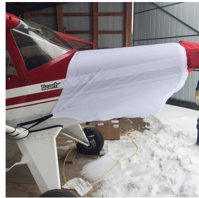
Bearhawk Engine Cover (test fit), Insulated Prop Cover
