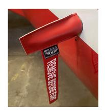
Cessna 501 Angle of Attack Transducer Cover
