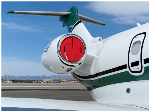
Embraer S A EMB-545 Engine Inlet & Exhaust Plug Set (folding type)
