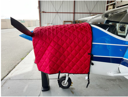
Insulated Hangar Blanket on Cessna 182
