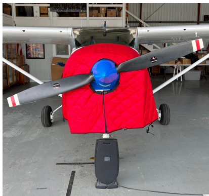
Insulated Hangar Blanket on Cessna 182
