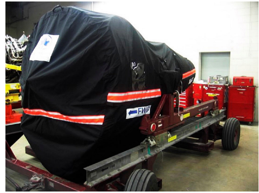
CFM-56-5A/5B Off-link Engine Shipper/Transport cover, w/ Exhaust Cone, fully enclosed
