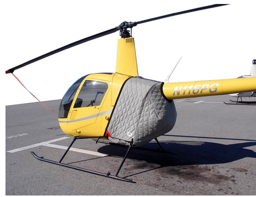
Robinson R-22 Light Weight Travel Cover Robinson R-22 Insulated Engine Cover (also covers bottom) & Front Blade Tie-down
