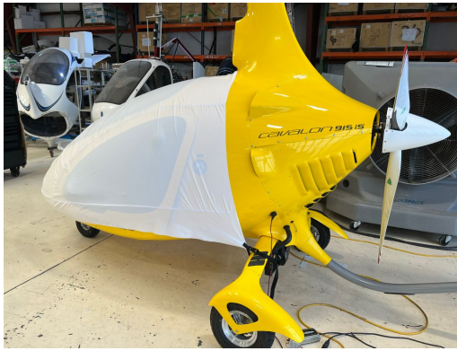
Autogyro Cavalon Canopy/Nose Cover, test fit cover
