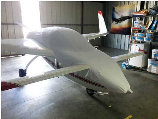
Cozy Canopy/Nose/Engine Cover, test fit cover
