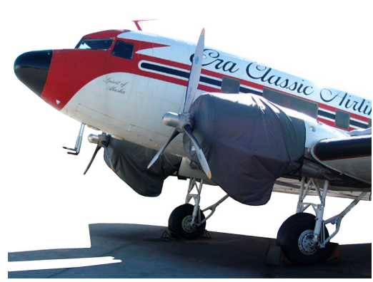
Engine Covers are available in either standard or insulated designs.
