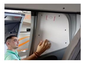
Airbus Helicopter EC130 B4 Side Window Heatshields
