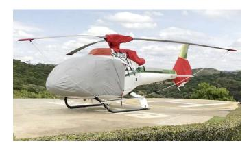
EC130 Bubble, Intake, Exhaust, Rotor Hub & Tailfan Covers
