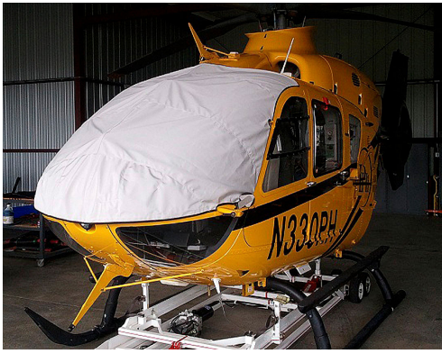
EC-135 Windshield/Skylights Cover, pinches in door jambs
