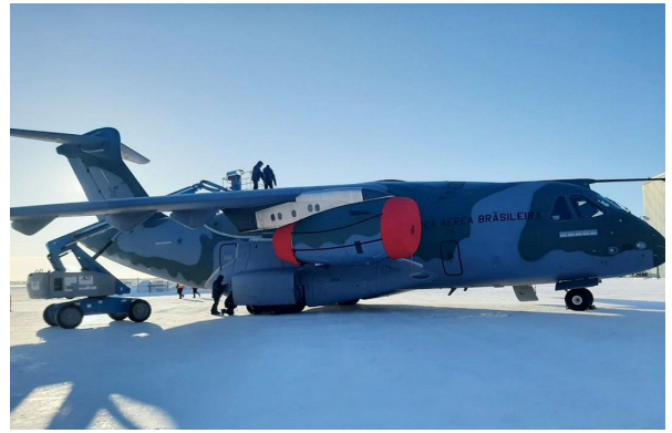
Embraer C-390 Millennium Intake/Exhaust Covers
