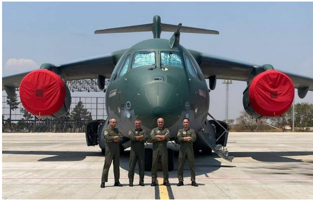
Embraer C-390 Millennium Intake/Exhaust Covers
