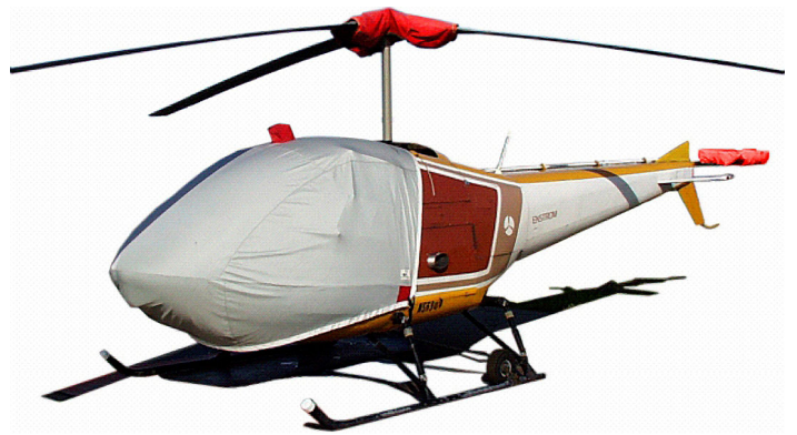
Enstrom 280FX Bubble, Main Rotor Mast, Tail Rotor Covers on Enstrom F280FX
