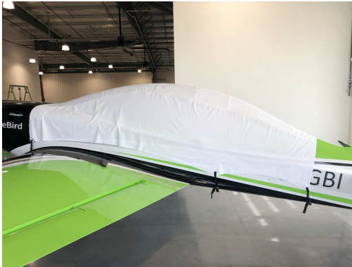
Game Composites GB-1 Canopy Cover, test fit cover
