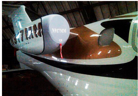
Phenom 100 Intake/Exhaust Cover, "Bikini" Type
