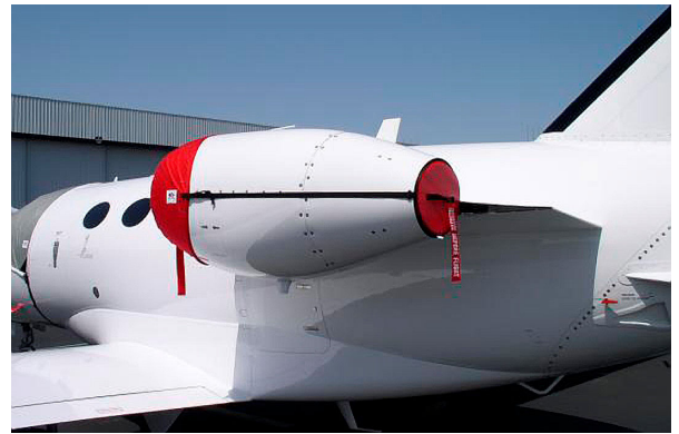
Cessna Mustang Intake/Exhaust Plug Set
