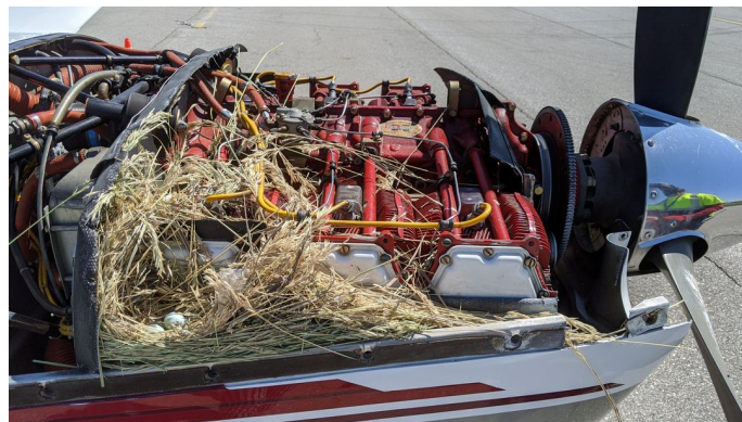
Piper PA-18 Super Cub Engine Inlet Plugs ENGINE PLUGS PREVENT BIRD NEST FOD. Piper Saratoga Engine Cowling Bird's Nest
