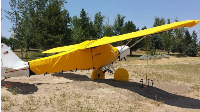
Piper PA-18 Super Cub Extended Canopy Cover, Wing & Tire Covers Cub Crafters CC19 Oversize Tire Covers, test fit cover
