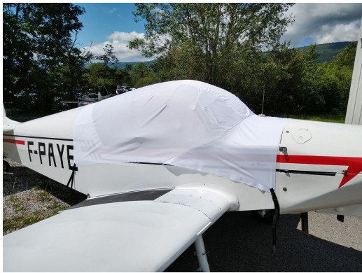
Jodel D113V Canopy Cover, test fit cover
