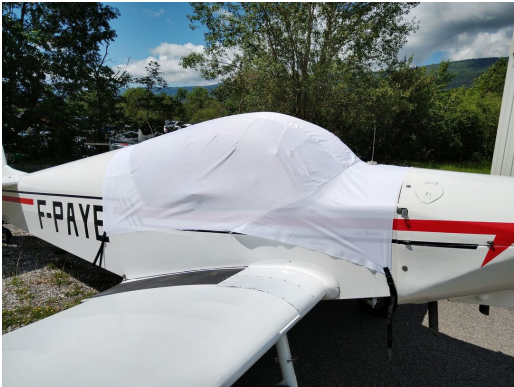
Jodel D113V Canopy Cover, test fit cover
