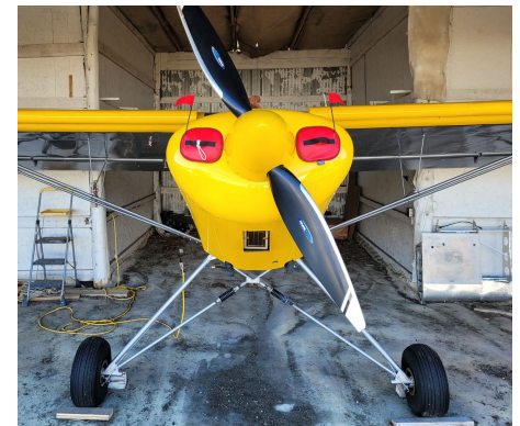
ENGINE PLUGS PREVENT BIRD NEST FOD. Piper Saratoga Engine Cowling Bird's Nest Preceptor STOL King Engine Plugs
