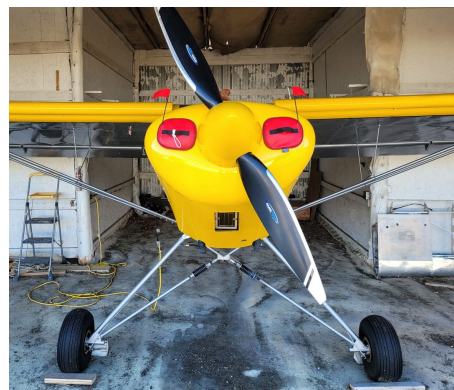
ENGINE PLUGS PREVENT BIRD NEST FOD. Piper Saratoga Engine Cowling Bird's Nest Preceptor STOL King Engine Plugs
