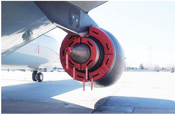
RC-135W Bypass Vent and Exhaust Plugs
