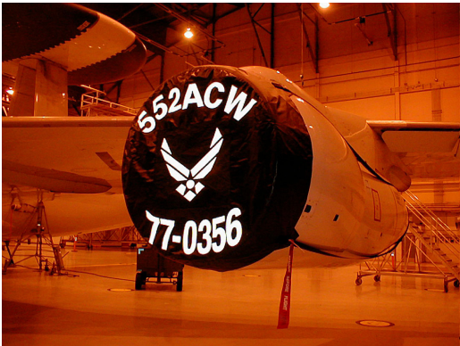
Intake/Exhaust Covers, soft type, TF-33 Engines
