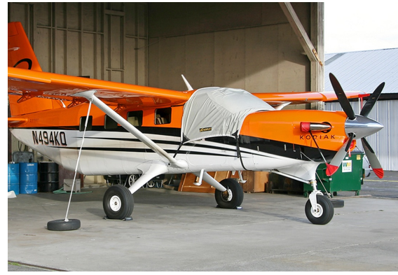
Quest Kodiak Windshield Cover, Prop Tie/Exhaust Covers, Engine Inlet Plugs & Pitot Cover
